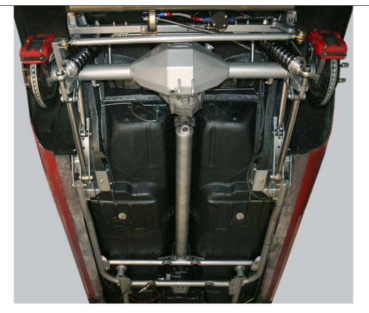
The finished project. This particular install utilized the 2 inch inset mini-tub frame brackets, the optional subframe connectors, driveshaft loop cross-member, Curries fabricated F-9 housing, aluminum adjustable coil-over's and Wilwood 13 inch disc brake kit with red 4 piston calipers.
